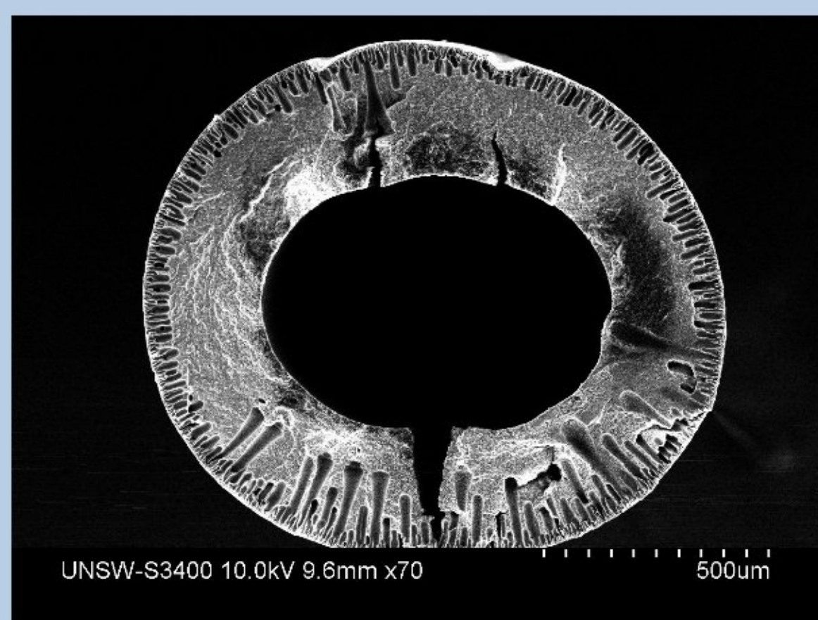
Cross section of previous hollow fibre indicating foulant has not penetrated pore structure.
