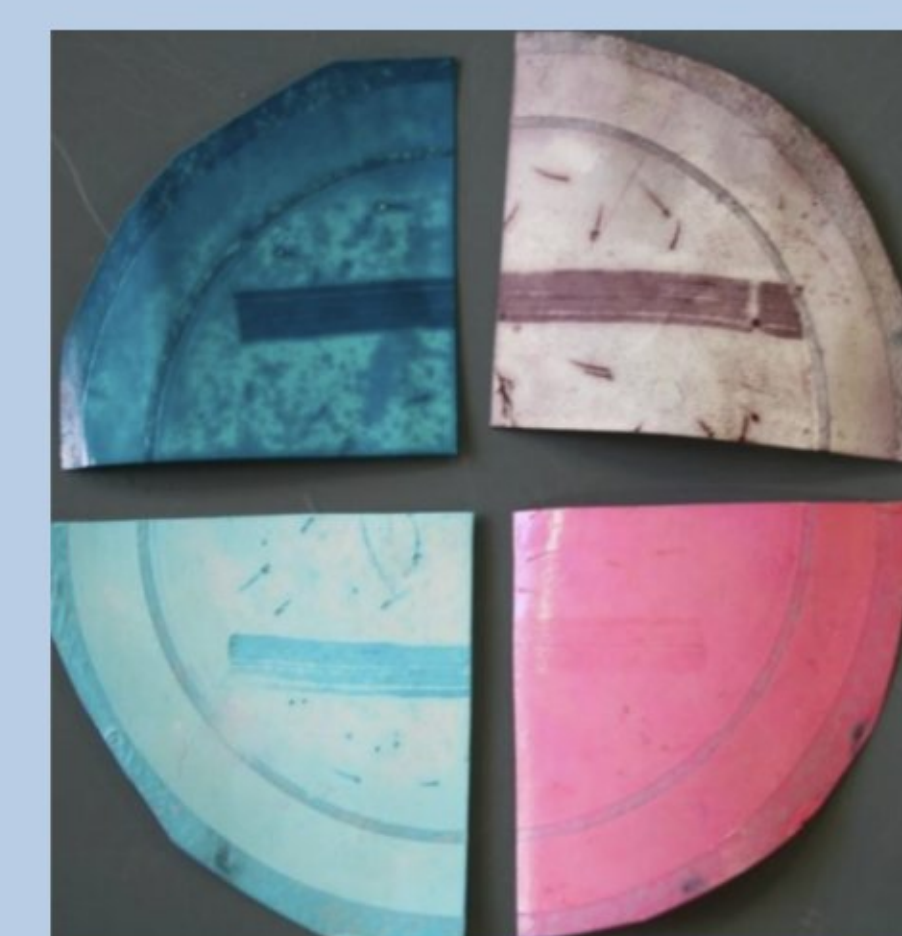
Membrane damage illustrated using different colour dyes.
